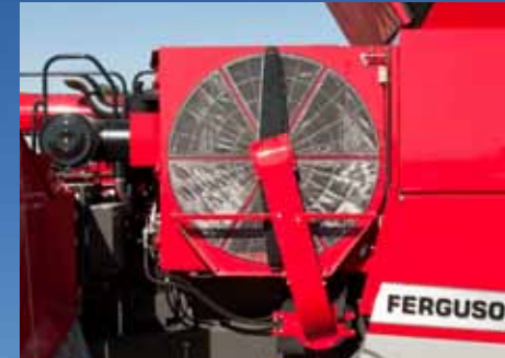
The hydraulically-driven vacuum wand removes chaff and debris from the cooling system and engine air intake for hours of harvesting without system maintenance.
