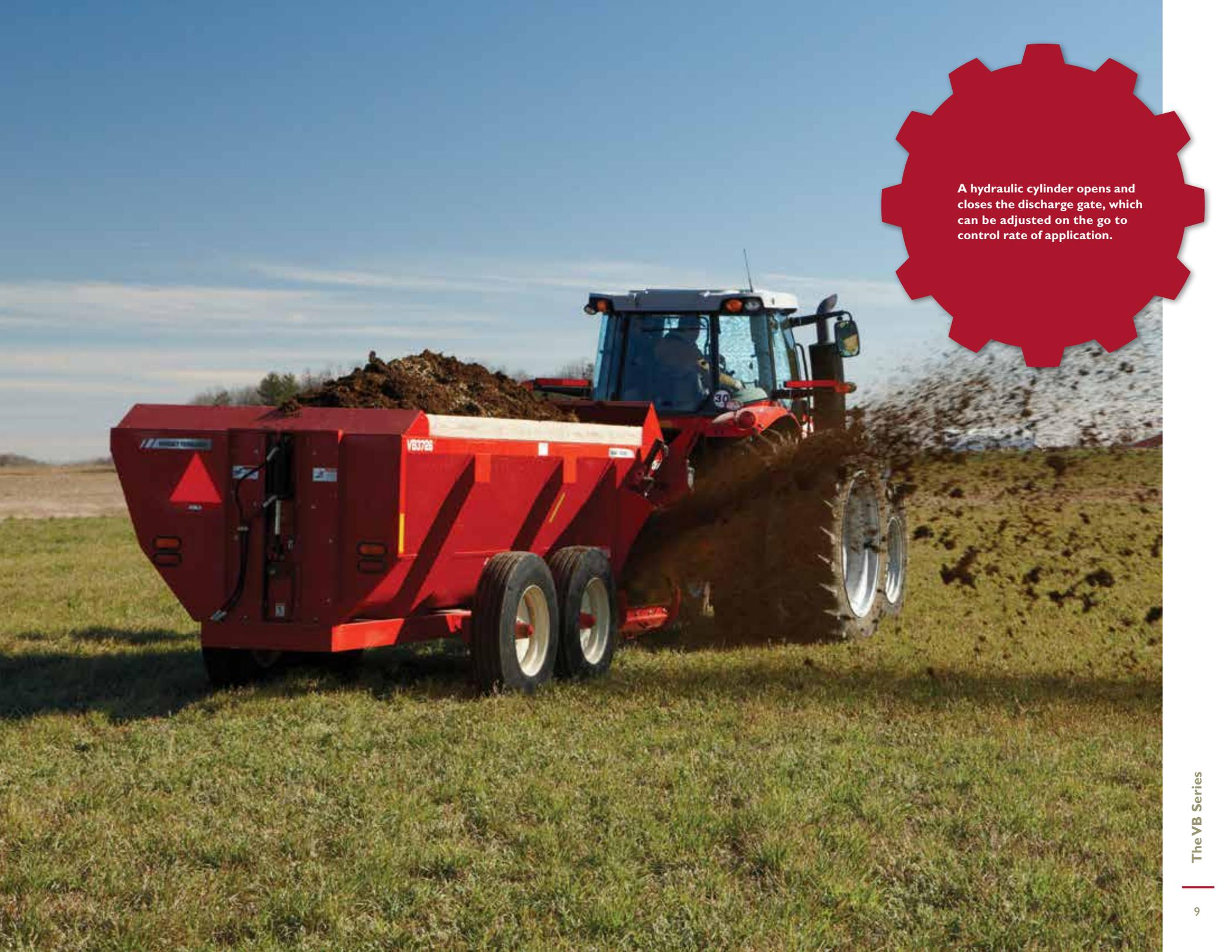
A hydraulic cylinder opens and closes the discharge gate, which can be adjusted on the go to control rate of application.
