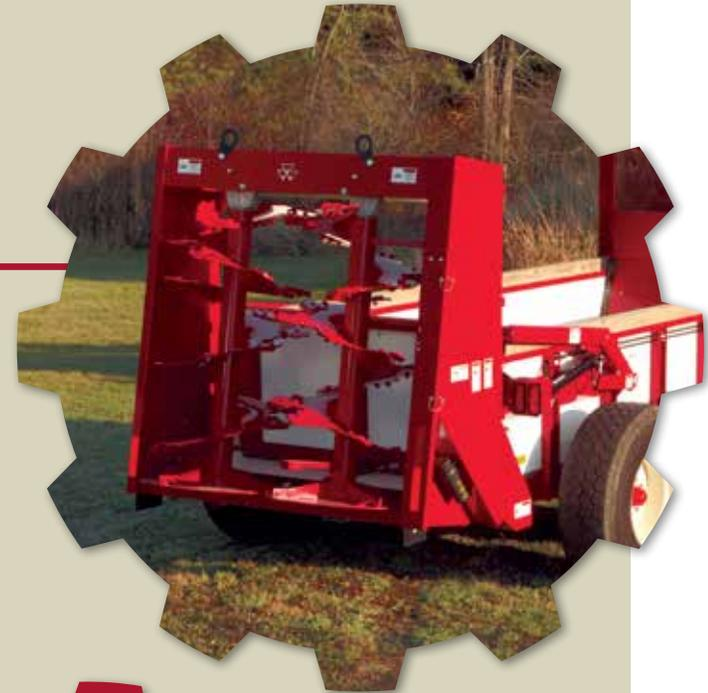
Beater gearboxes on the vertical beater assembly are mounted at the top of the assembly rather than the bottom, to avoid damage.
