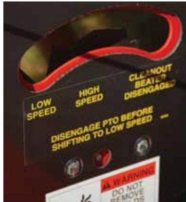
Two-speed apron drive is standard equipment on most models except the SP3735 & SP3748. These two models come standard with the Electric-over-hydraulic variable speed drive.
