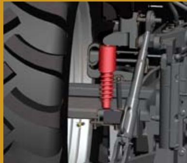
The cab suspension system uses new silent block bushes at the front of the cab and a pair of spring assisted shock absorbers mounted at the rear. Although vertical damping is the key attribute, damping is actually provided in three dimensions with a panhard rod providing lateral stability.
